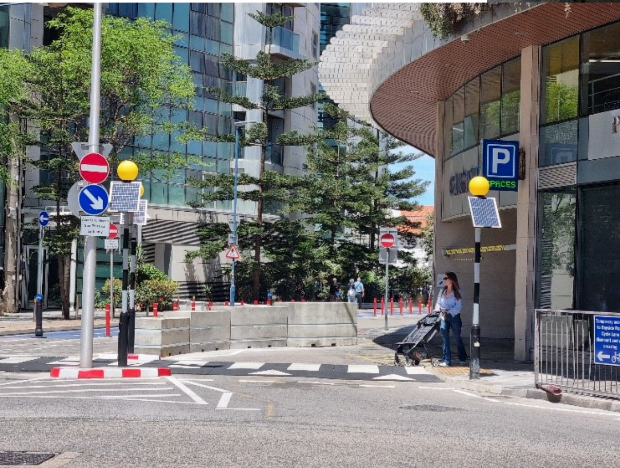
Solar powered Belisha Beacons at Glacis Road crossing.
