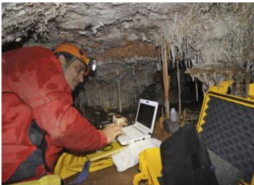
GONHS Cave Science Unit in action: John Paul Latin downloads drip discharge and temperature data in Straw chamber (Ragged Staff Cave system).
