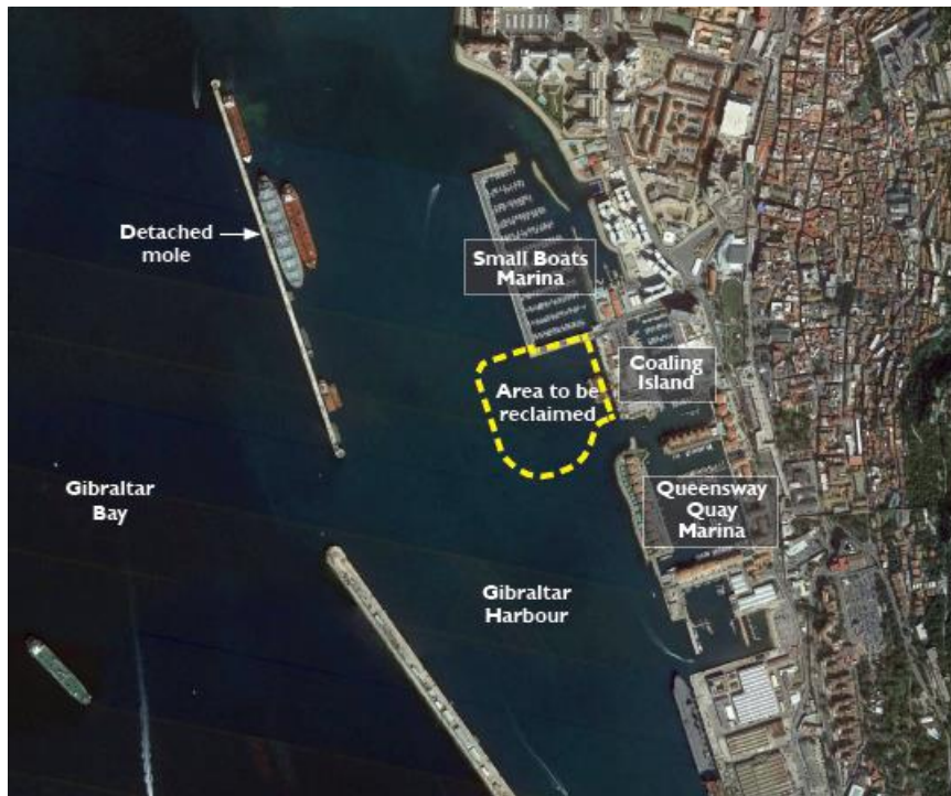
Figure 3-3: Proposed Coaling Island Reclamation Works.
