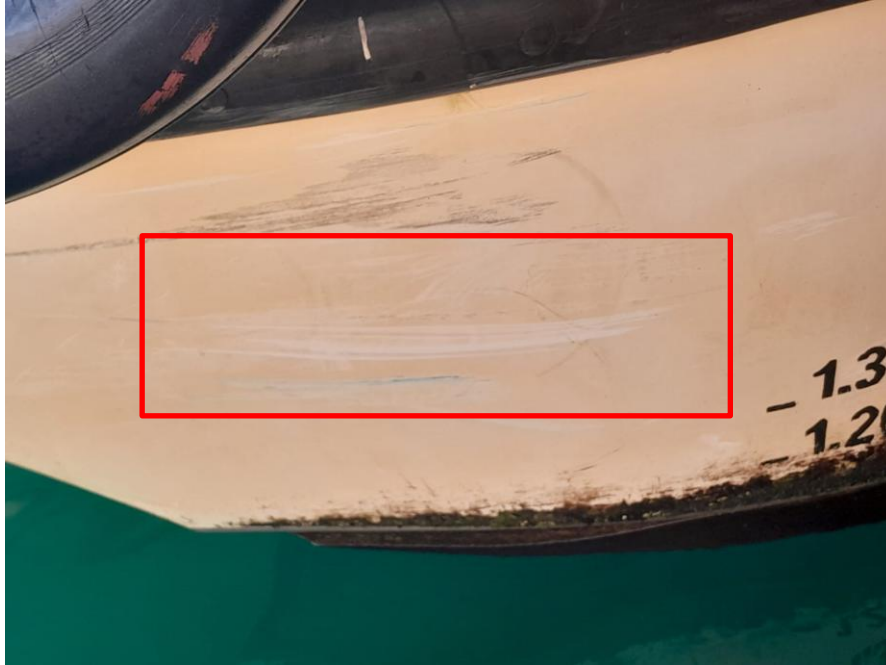
Fig. 8 – Damage sustained to SAMMY ONE Port Hull
