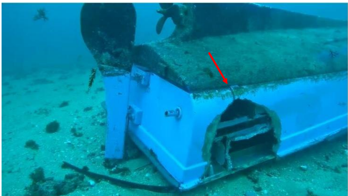
Fig. 9 – Damage sustain to Keith Port side quarter
