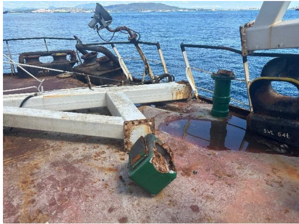
Figure 6 - General View of davit support structure collapsed & aft peak tank air pipe damaged / fractured
