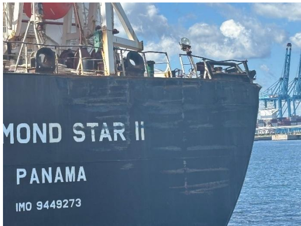
Figure 11 - General View of aft transom plating deformed / buckled
