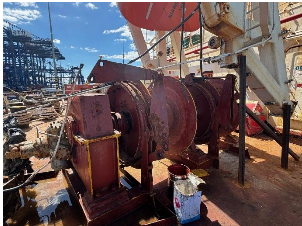
Figure 8 - General View aft deck deformed & buckled / Mooring windlass brake structural damage
