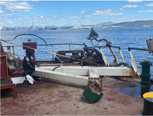
Figure 6 - General View of davit support structure collapsed & aft peak tank air pipe damaged / fractured
