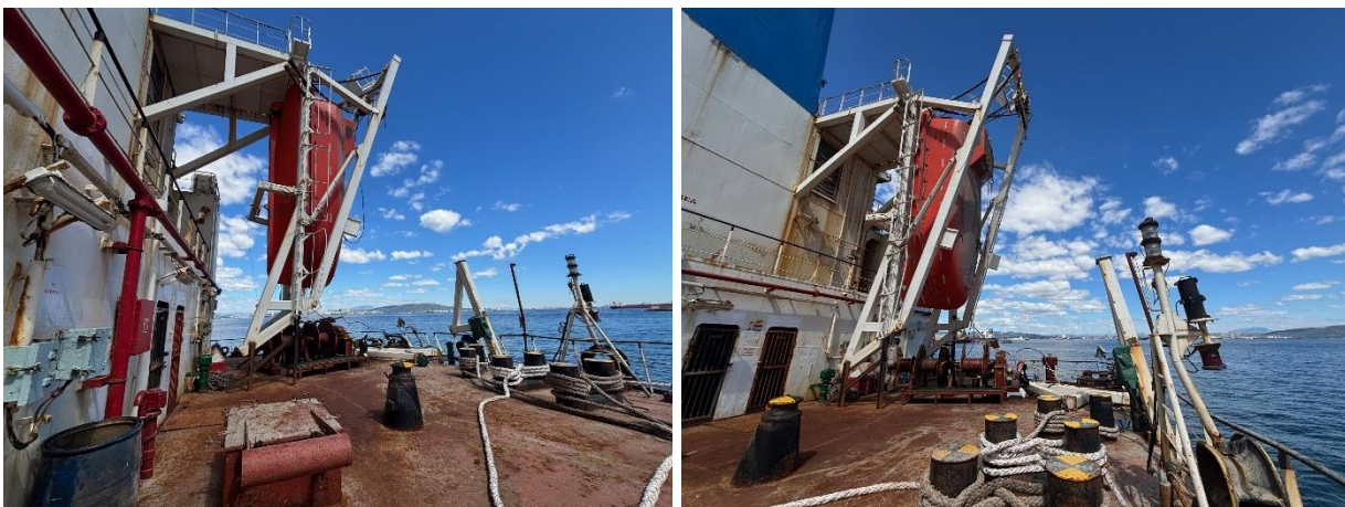
Figure 5 - General View of freefall lifeboat & davit secured by welding after damage
