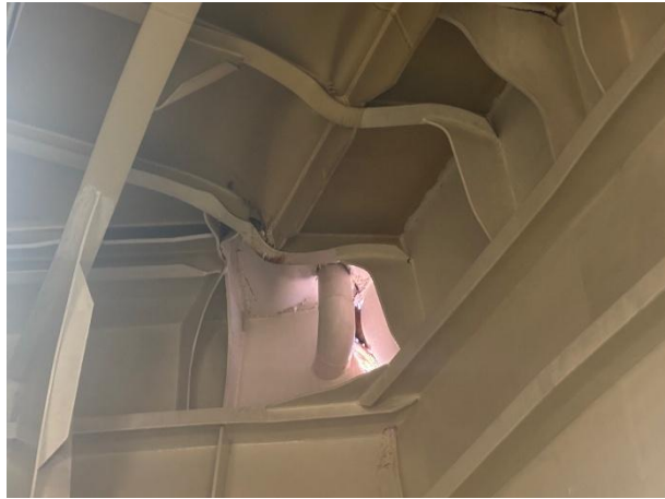
Figure 9 - General View internally of aft Stbd side quarter deformed / buckled / holed
