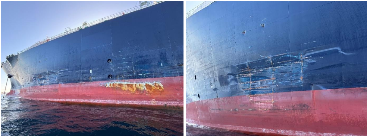
Figure 3 - View of Port side hull damage
