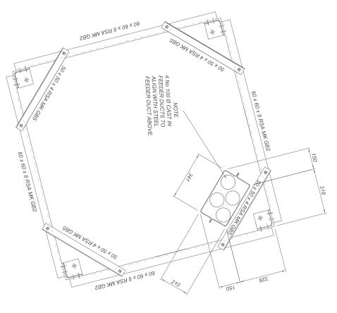
LAYOUT OF CAST IN DUCTS - APPLIES TO ANY LEG
