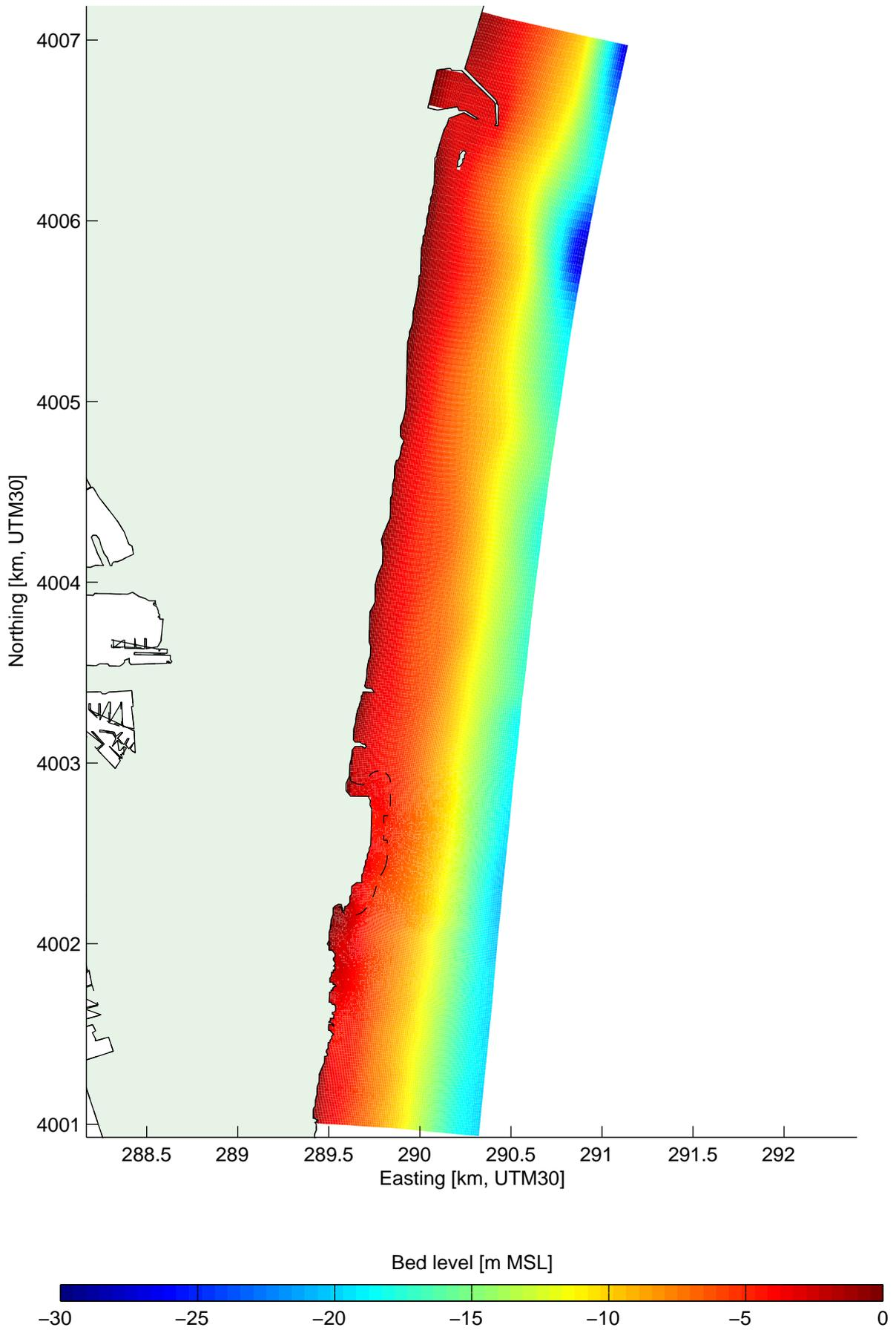
Bathymetry for the detailed domain of the flow model
