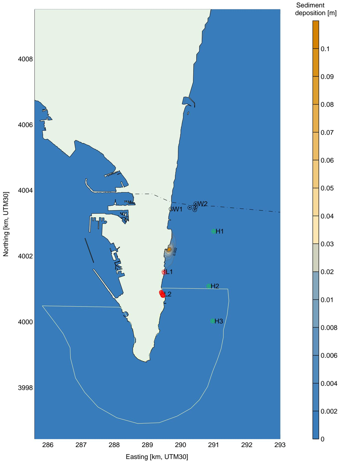
Deposited sediment thickness due to scenario 1a
