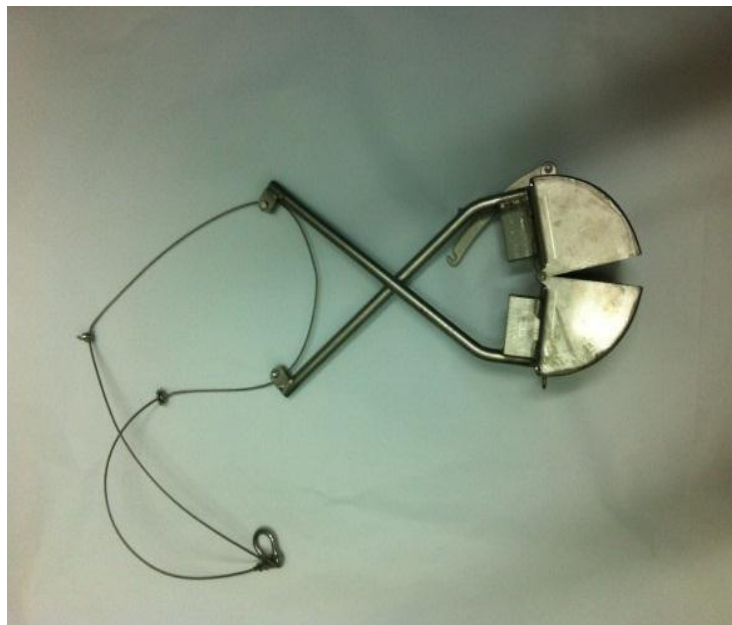
Figure 2.2 Van Veen Grab used for collecting sediment samples
