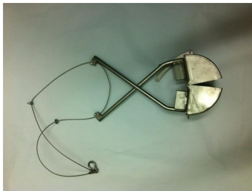
Figure 2.2 Van Veen Grabs used for collecting sediment samples.
