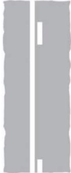
Overtaking allowed on broken line side
