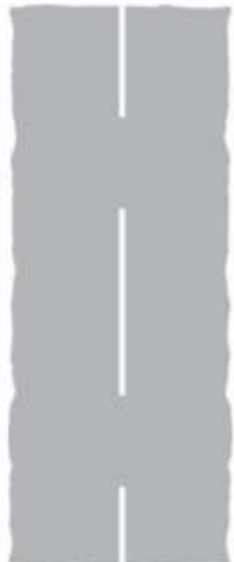
Hazard Warning Line
